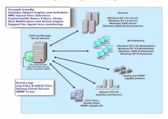
ELM Log Manager is a 32-bit, multi-threaded application designed to monitor Windows NT, Windows 2000 and Windows XP computers in real-time. It is a client/server application that automates a variety of the administrative functions required for monitoring and managing Windows-based servers and TCP/IP systems and devices. It's multi-layered architecture enables you to deploy ELM Log Manager in a manner that suits your organization's needs.
