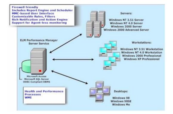
ELM Performance Manager is a 32-bit, multi-threaded application designed to monitor and collect performance data and WMI data from Windows NT, Windows 2000, and Windows XP computers in real-time. It's multi-layered architecture enables you to deploy ELM Performance Manager in a manner that suits your organization's needs.
